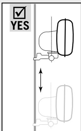
Using oscillating function when the fan is leaning forward more than 15 degree result in damaging the motor and shorter the lifetime of your product.
